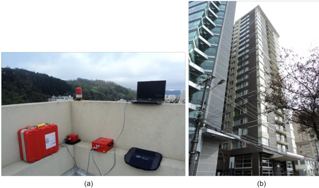
Figure 3. (a) Measurement in the top of the Concepto Urbano building. (b) Concepto Urbano building
