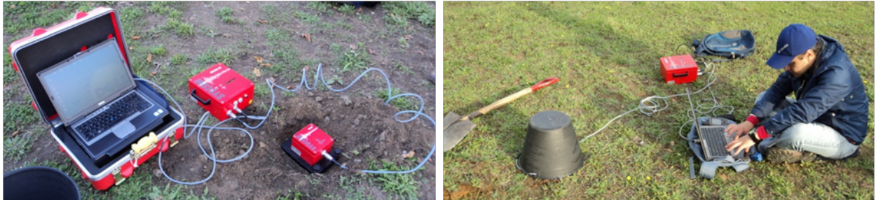
(a) (b) Figure 1. (a) Velocity sensor. (b) Final view of the installation of the entire system
